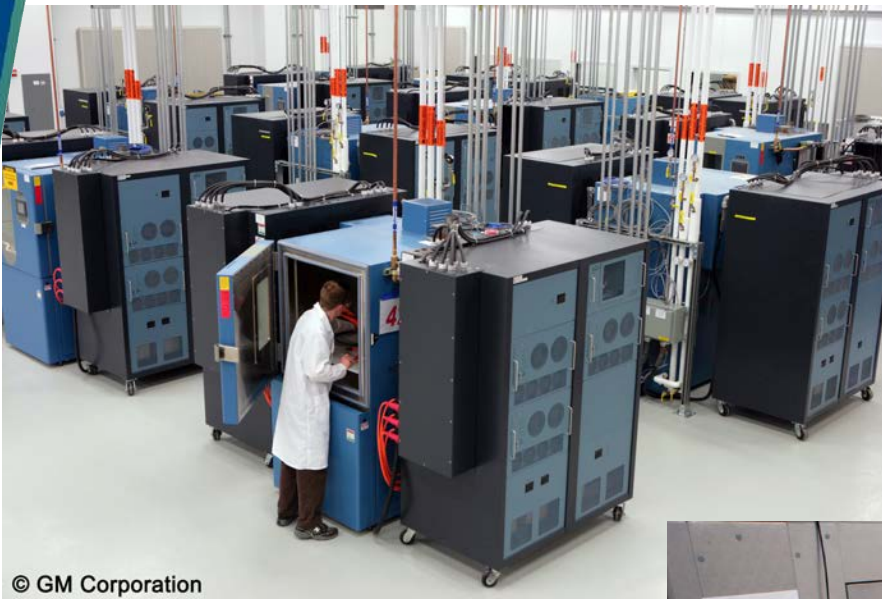
CSZ reach-in and walk-in chambers featured at GM Battery Test Laboratory.
